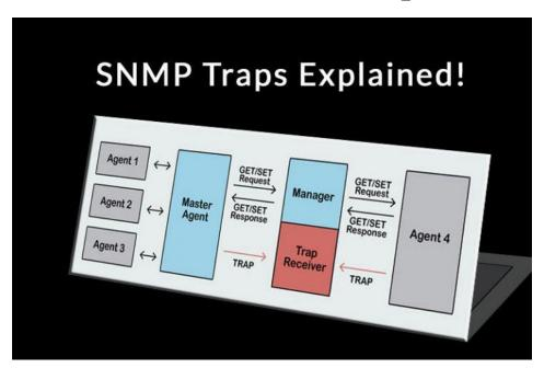
Simple Network Management Protocol (SNMP) is used by different devices (Routers, Switches, Printers, etc.) on the network to check each other's activity and communicate critical information.
